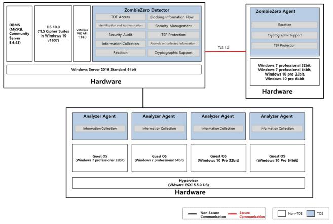
[Figure 3] Logical Scope of TOE
